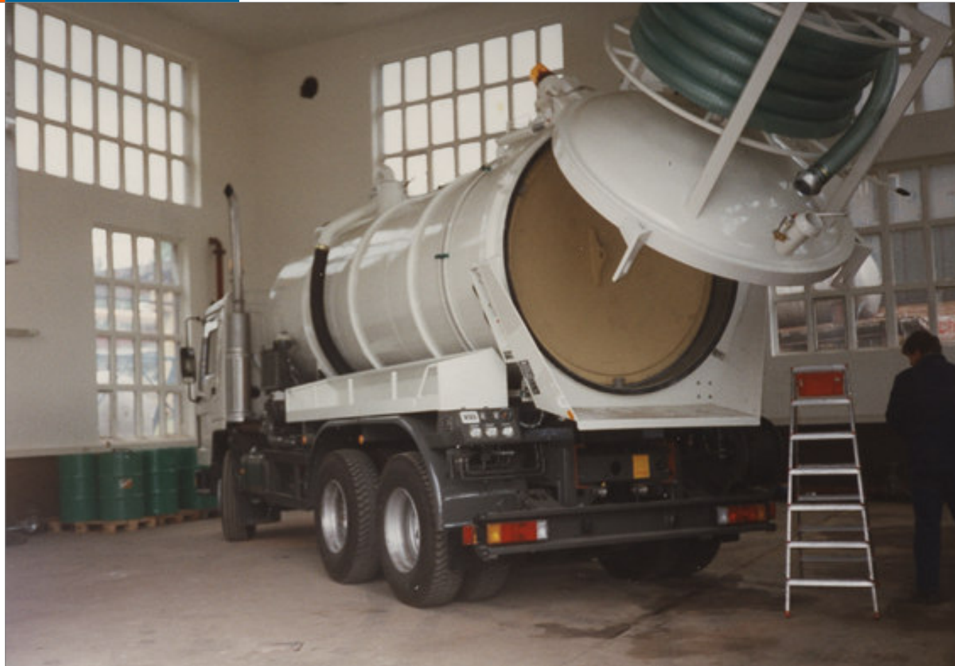
heat cured coating Si 57E Truck container
