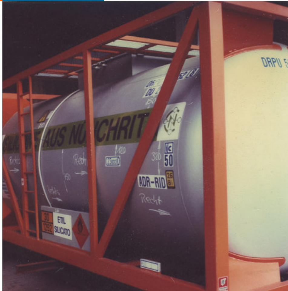
heat cured coating Si 14E of road container
