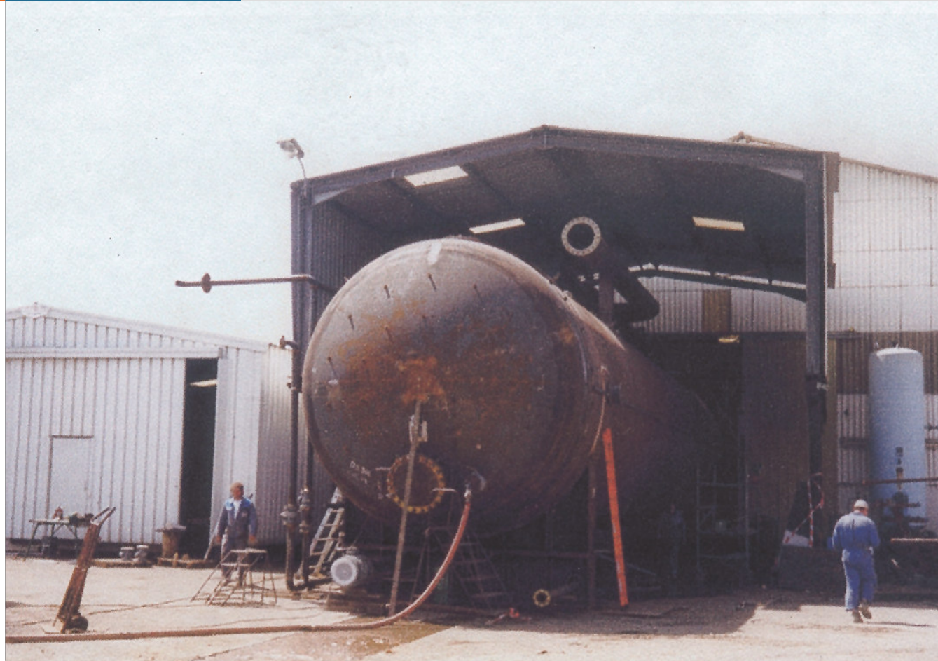
road container internal coated with SI14E
