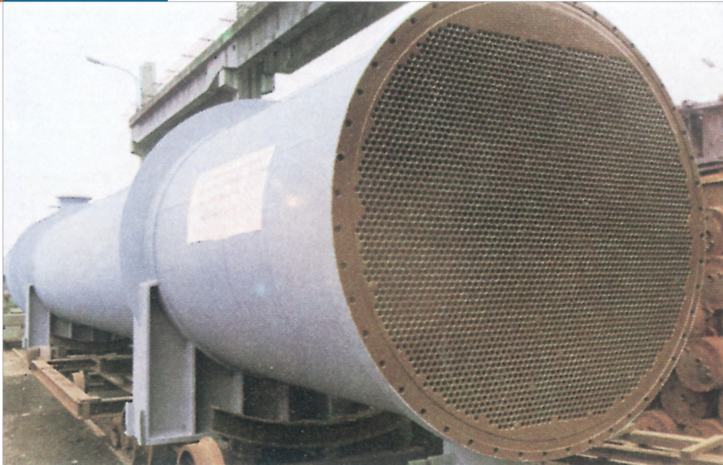
condenser (tube-side coated), ordered by BASF AG, Germany
