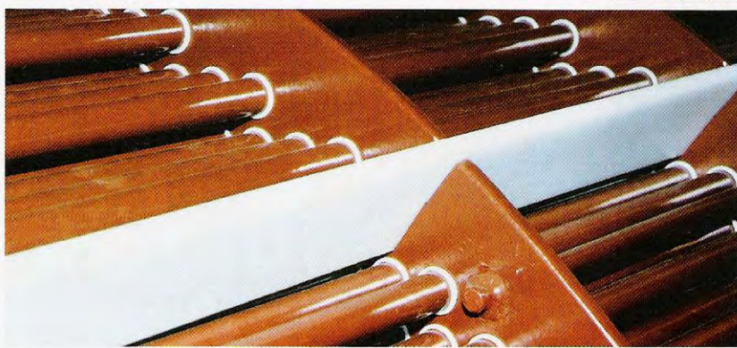
Heat exchanger for the chemical industry, shell side coated with the SAEKAPHEN coating material Si 57 E
